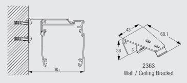
The ceiling fixing with the Bracket 2363 is according to the ceiling fixing with the Bracket 2521.
