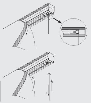
With the new developed cord release mechanism, taking down of the fabric becomes very easy.
