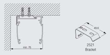
Ceiling / Wall fitting with bracket 2363
