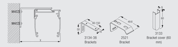
Brackets feature thread for screw M4 x 6 for fixing the Bracket 2521.
