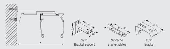
Brackets feature thread for screw M4 for fixing the Bracket 2521.
