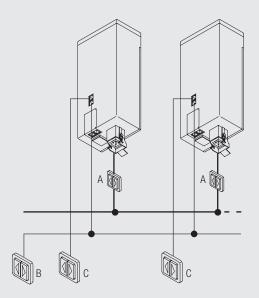
A: High voltage current 230V/115V mains individual B: Low Voltage (potential-free) simultaneous C: Low Voltage (potential-free) individual
