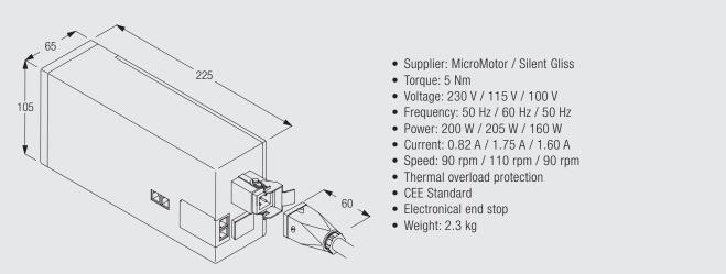
The Silent Gliss 5360 motor is an interference-free asynchronous motor, designed to offer advanced features. Multiple motors can be individually and/or simultaneously controlled with cost effective and simple low voltage wiring (no relays). The entire motor is hidden behind the curtain.
